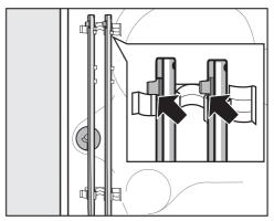
Secure the transit bars to the back of the washing machine. Make sure the top catch is located above the holder.
